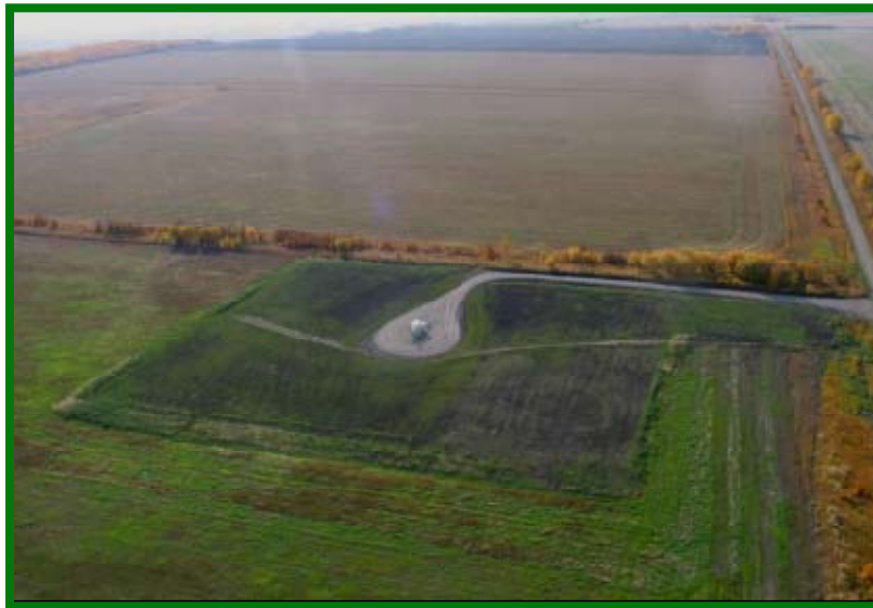
This well site has been 'tear dropped', enabling farming to continue. Note access is along the field edge to minimize disruption to cultivation.
