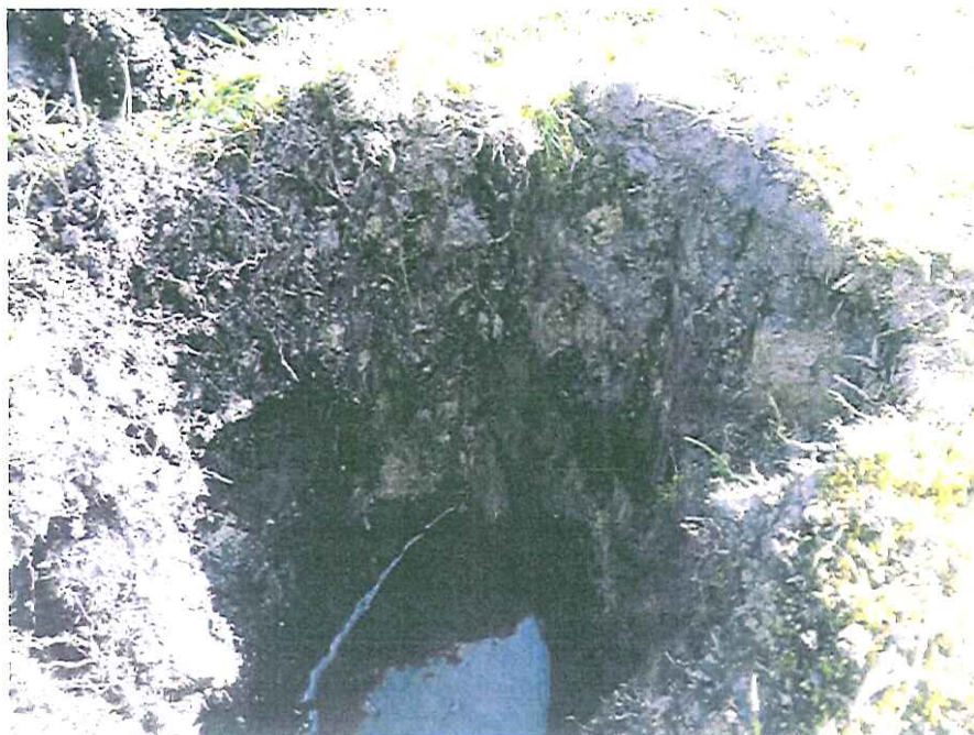
Photo 2. Soil profile showing veneer of silt loam from an earlier fill placement and underlying black, well-humified organic horizons. This is a Typic Humisol.
